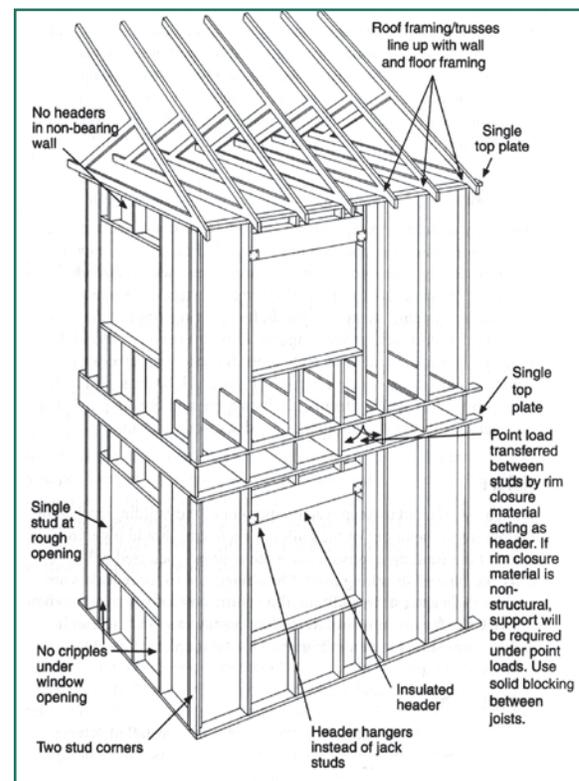
Diagram showing Advanced Framing details<sup>8</sup>
