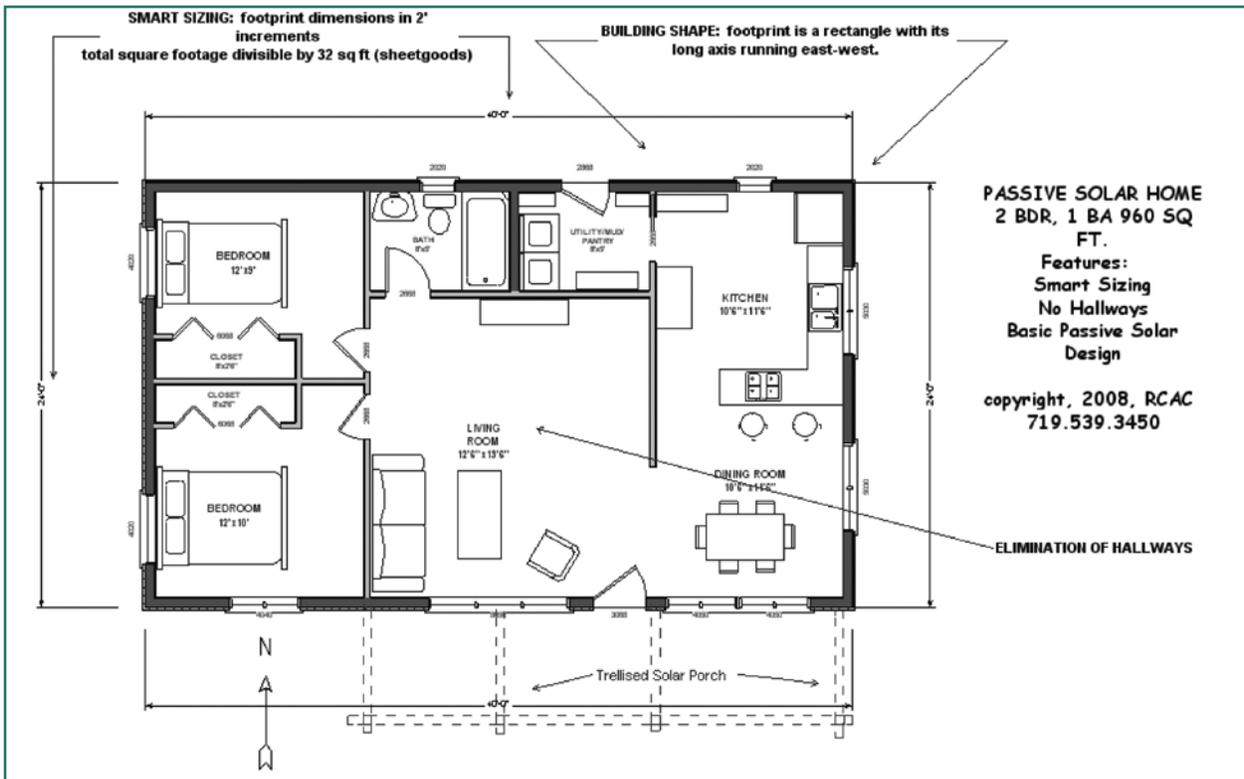
Passive solar home floor plan illustrating smart sizing, building shape, daylighting and hallway elimination
